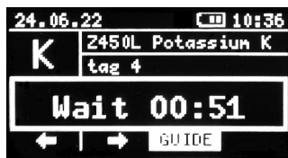
Switch on the test guide system Press the GUIDE context button and follow the instructions displayed on the screen.
