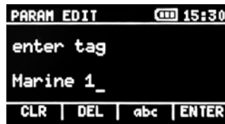
Editing tags list MAIN MENU → Sample Tags Choose a tag from the displayed list and press the EDIT context button.
