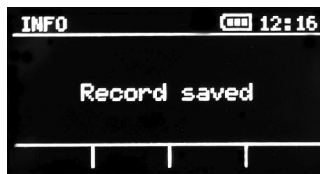
Record the result Press the REC context button to record the displayed result in the device's log.
