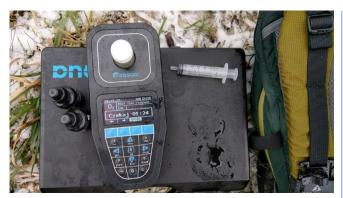
Alternative to classic oxygen meters The ability to measure the concentration of dissolved oxygen using the Exaqua photometer is a great alternative to classic oxygen meters.
