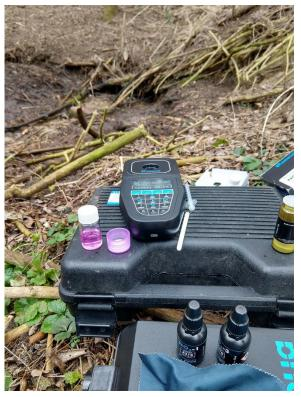
**Routine measurements from the spring** Routine measurement of nitrate ion concentration in water from the spring in the Pilica River valley.
