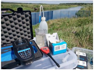
**Field exercises in full sunlight** We used the Exaqua PRO3 photometer during field exercises for chemical analysis of water samples from the Krzna River. The device is doing great even in full sunlight.
